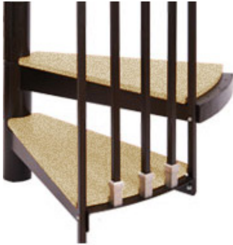
3/4" Plywood Tread Coverings Used as an underlayment for carpeting.
